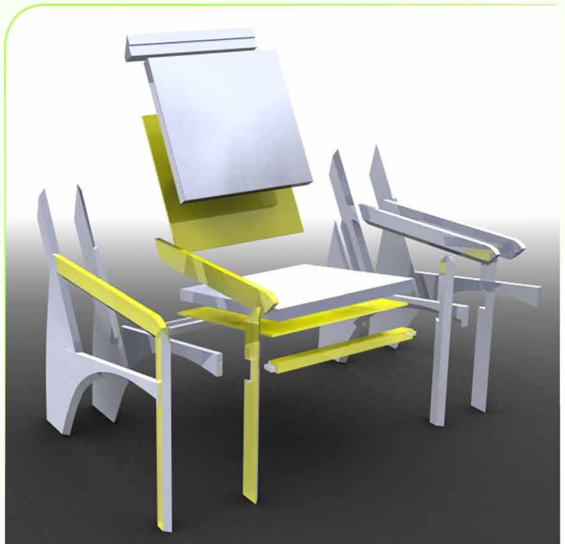
Exploded Solid Works model of the production chair
